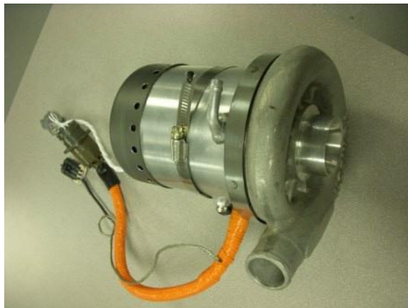
Figure 2. Electronic Supercharger (ESC), Integral Motor/Compressor System
