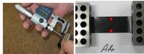
Figure 9. Top Foil overall thickness measurement (left) and measurement locations (right)
